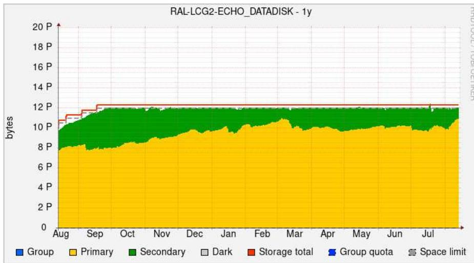
Figure-10: The available and used disk capacity at the UK Tier-1 for ATLAS.
